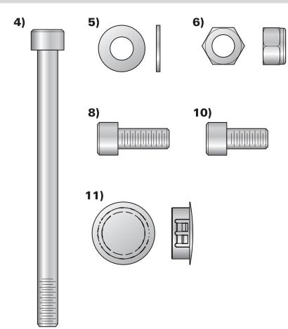
LOOSELY assemble the LEFT UPRIGHT (2) and RIGHT UPRIGHT (3) to the CROSS BRACE (3) using four M10 X 135mm BOLTS (4), eight 3/8" SAE WASHERS (5), and four M10 NYLOCK NUTS (6) as shown.
