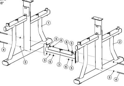
Assemble ARM PAD SUPPORT (7) to the LEFT UPRIGHT (2) and RIGHT UPRIGHT (3) using four M10 X 25mm BOLT (8), six 3/8" SAE WASHERS (5) and two M10 NYLOCK NUTS (6) as shown. Tighten all BOLTS securely.
